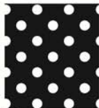
Hole Diameter 3.0 Pitch 10.0, % Open Area 8.2
