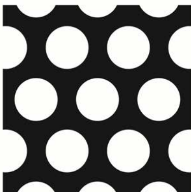
Hole Diameter 18.0 Pitch 26.0, % Open Area 43.4
