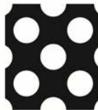
Hole Diameter 8.0 Pitch 12.0% Open Area 34.9
