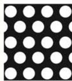
Hole Diameter 5.0 Pitch 8.0, % Open Area 35.4
