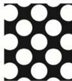
Hole Diameter 7.0 Pitch 9.0, % Open Area 54.9
