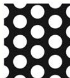
Hole Diameter 6.0 Pitch 9.0, % Open Area 40.3
