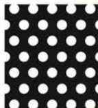
Hole Diameter 3.0 Pitch 6.0, % Open Area 22.7
