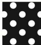
Hole Diameter 5.0 Pitch 10.0, % Open Area 19.6
