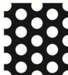
Hole Diameter 5.0 Pitch 8.0, % Open Area 35.4
