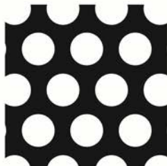
Hole Diameter 10.0 Pitch 15.0, % Open Area 40.2
