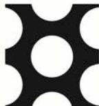
Hole Diameter 13.0 Pitch 18.0, % Open Area 47.3
