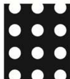
Hole Diameter 8.0 Pitch 16.0% Open Area 19.6
