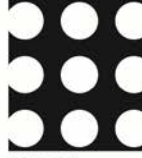
Hole Diameter 10.0 Pitch 50.0% Open Area 3.1
